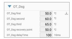
**OT-Dsg First** - First-level warning of Battery discharging over temperature. When the temperature of battery exceeds the critical value during charging, the first-level warning of Battery discharging over temperature will be generated.
