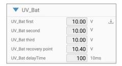
**UV-Bat First** - First-level warning of Battery pack undervoltage. When the total voltage of the battery pack is lower than the critical value, the first-level warning of battery pack under-voltage will be generated.
