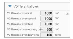
**VDifferential over First** - First-level warning of battery voltage differential When the battery voltage differential exceeds the critical value, the first-level warning of battery voltage differential will be generated.
