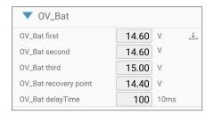
**OV-Bat First** - First-level warning of Battery pack overvoltage. When the total voltage of the battery exceeds the critical value, the first-level warning of battery pack over-voltage will be generated.
