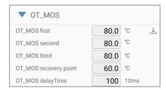
**OT-MOS First** - First-level warning of MOS over temperture. When the MOS temperature exceeds the critical value during battery charging/discharging, the first-evel warning of MOS over temperture will be generated.
