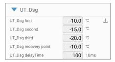
**UT-Dsg First** - First-level warning of Battery discharging low-temperature. When the temperature of battery is lower than the critical value during charging, the first-level warning of Battery discharging low-temperature will be generated.
