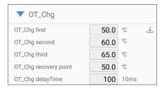
**OT-Chg First** - First-level warning of Battery charging over temperature. When the temperature of battery exceeds the critical value during charging, the first-level warning of Battery charging over temperature will be generated.
