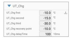
**UT-Chg First** - First-level warning of Battery charging low-temperature. When the temperature of battery is lower than the critical value during charging, the first-level warning of Battery charging low-temperature will be generated.
