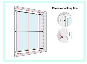
This is the measurement you need to take if you want your blind to fit inside the window recess. Measure the full width and height of the recess – leave deductions to our experts. You will get a blind ready to fit inside the recess perfectly.
