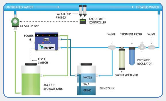
A Service Wing technician installs all of our anolyte generators on-site, and our delivery time is 1-2 weeks. The space needed for our generators is approximately 4'x8'. The customer will also need to provide 220V power, water line, drain line, storage tank for disinfectant, and Morton Water Softener Pellets.
