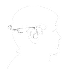
Adjust the angle of the speaker to face your ear canal until you receive the desired sound clarity and fit.
