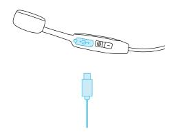
Plug in the included charging cable. The LED will be red when charging and turn blue when fully charged.
