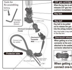
CO<sup>2</sup> gas cartridge When the key box is activated, the gas cartridge releases  ${\rm CO^2}$  gas into the airbag (to each air
