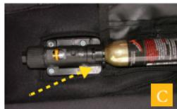
**C** When the retention lug on the bayonet fitting reaches the right hand side of the location slot (shown by the yellow arrow in the picture), you will feel the cartridge loosen in the trigger body.
