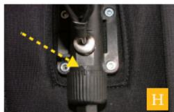
H Finish tightening the cap with the Allen key, until the lip of the spring tension cap is flush with the trigger body and the markers on the trigger body and spring tension cap line up as shown by the yellow arrow.
