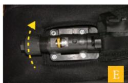
E Loosen the spring tension cap with the Allen key provided, turning it in the direction shown by the arrow, until the spring drops out of sight below the bottom of the release pin aperture of the trigger body.
