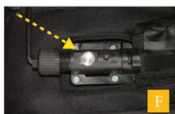
F With your finger or with the allen key, push through the trigger aperture to move the piston back to its location. Ensure the recess of the silver piston is aligned with the hole in the centre of the trigger casing - as pictured.
