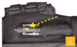
**A** This is how the trigger looks after activation. The release pin and lanyard have detached, the piston has slid towards the cartridge and the spring (marked with a yellow arrow) is visible.
