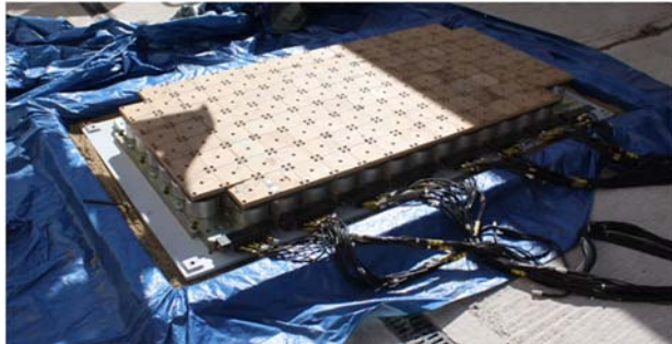
Fig. 5. Load cell wall, showing the array of 123 load cells.
