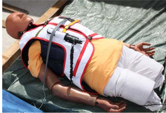
Fig. 7. ATD wearing body protector and air jacket positioned on the load cell array prior to Test 1.
