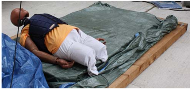
Fig. 10. ATD wearing body protector only, positioned on the load cell array prior to Test 2.
