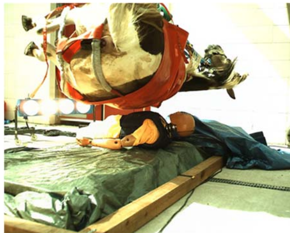
Fig. 2. Rear three-quarter view of Test 2 (non-inflatable body protector only).
