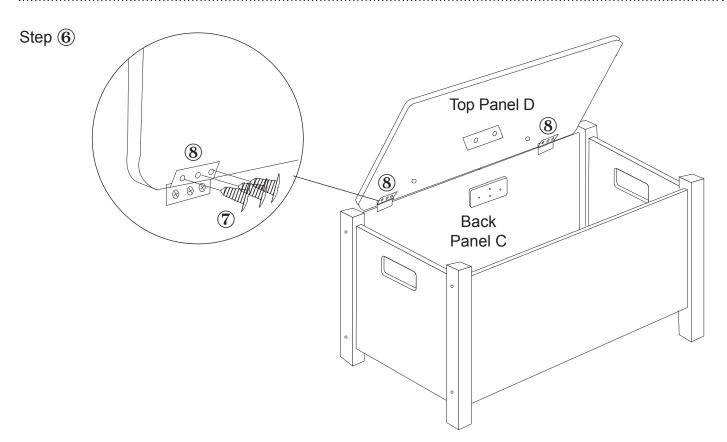
Secure 2 x Hinge 8 to Top Panel D using 6 x Screw 7.
