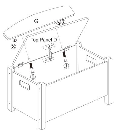
Insert 2 x Bolt 3 into Panel G. **Align correctly.**Secure Panel G to Top Panel D using 2 x Screw 1.
