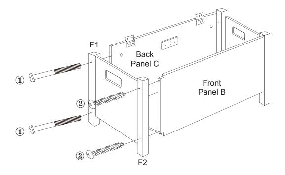
Secure F1 to Back Panel C using 2 x Screw 1. Secure F2 to Front Panel B using 2 x Screw 2.
