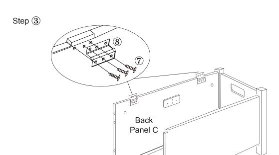
Secure 2 x Hinge 8 to Back Panel C using 6 x Screw 7.
