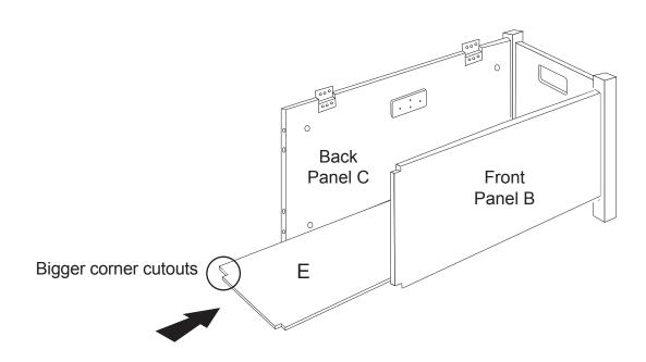
Insert Panel E. Ensure the bigger corner cutouts are at the back.
