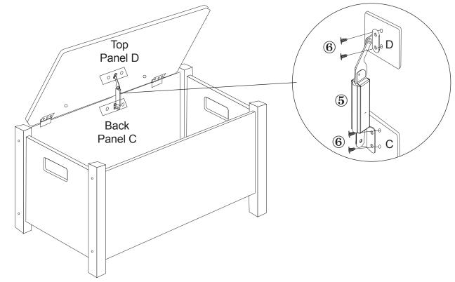
Secure Hinge 5 to Back Panel C using 2 x Screw 6. Secure Hinge 5 to Top Panel D using 2 x Screw 6.
