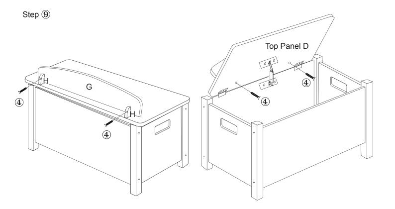
Secure 2 x Part H to Panel G using 2 x Screw 4. Lift Top Panel D and secure Part H to Top Panel D using 2 x Screw 4.
