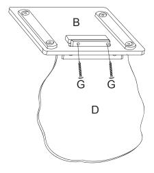
Secure Seat Back D to Seat B using 2 x Screw G. **REPEAT FOR OTHER CHAIR.**
