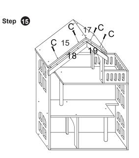
Use 2 x Screws C to secure Panel 15 to
