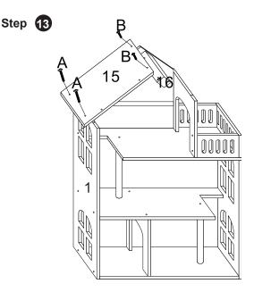
Use 2 x Screws A to secure Panel 15 to Panel 1.
