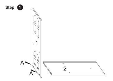
Secure Side Panel 1 to Panel 2 using 2 x Screws A.
