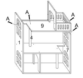
Use 1 x Screw A to secure Panel 9 to Support Column 4. Use Screws A to secure Panel 9 to side Panels 1 and 7.
