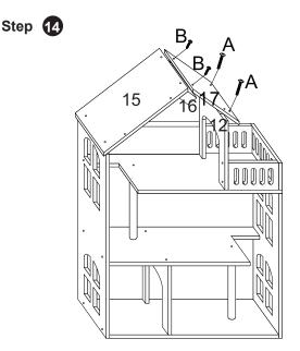
Use 2 x Screws A to secure Panel 17 to Panel 12.
