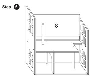
Insert Back Panel 8 in backside groove.
