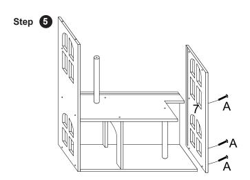
Secure Panel 7 on right side using 3 x Screws A.
