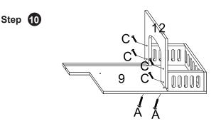
Secure Panel 12 to Panels 11 using 4 x Screws C. Secure Panel 12 to Panel 9 using 2 x Screws A.
