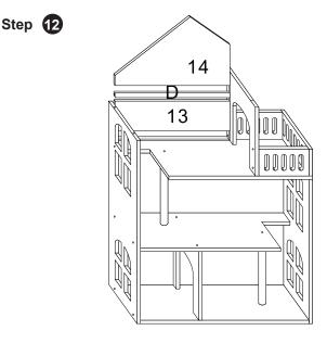
Insert Back Panel 13 in to groove. Attach Plastic Bar D to Panel 13. Insert Back Panel 14 in to Plastic Bar D.
