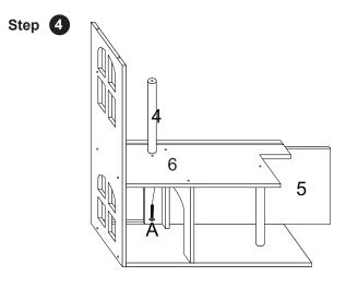
Insert Back Panel 5 in backside groove. Secure Support Column 4 to Panel 6 using 1 x Screw A.
