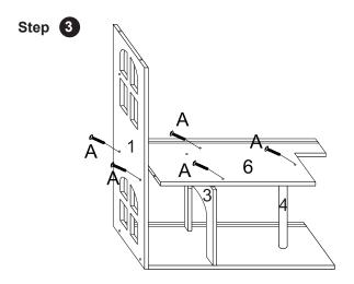
Use 2 x Screws A to secure Panel 6 to Side Panel 1.
