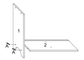
Secure Panel 1 to Panel 2 using 2 x Screws A.
