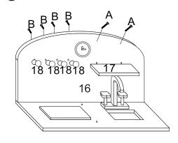
Secure 4 x Panel 18 (Utensil Hook) to Panel 16 using 4 x Screws B. Secure Panel 17 (Shelf) to Panel 16 using 2 x Screws A.
