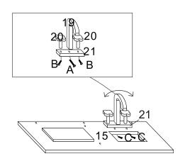
Secure Panel 19 (Tap Faucet) to panel 21 using 1 x Screw A.
