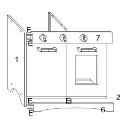
Secure Handle I to Panel 4 using 2 x Screw B. Secure Handle I to Panel 5 using 2 x Screw B. Use Screws D to secure Door Pins F and G to Panels 4 and 5.
