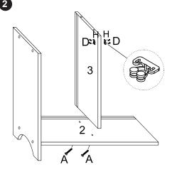
Use Screws D to secure Lock H (female hinge) to Panel 3.
