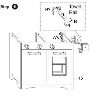
Secure Panels 10 and 11 to Panel 9 (Rail) using 2 x Screws B.
