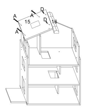
Put No.16 panel on No.11 panel, then use D screw to lock No.16 panel on No.15 panel, joint No.10 panel to No.15 panel, use A screw to lock No.15 panel on No.10 and 13 panel.
