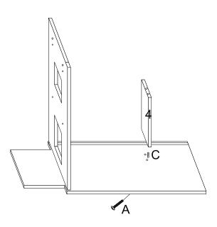
Insert C (wooden dowel) in No.4 panel bottom, join it to No.2 panel, use A screw to No.4 panel on No.2 panel.
