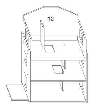
Insert No.12 panel in top backside groove.
