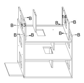
Insert B(female) in No.13 and 14 panel, use B(male) to across No.1 and 9 panel, to lock No.13 and 14 panel.
