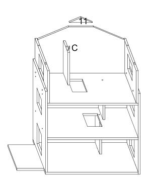
Insert C(wooden dowel) in No.10 panel top, put No.11 panel on No.12 panel top.
