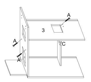
Insert C(wooden dowel) in No.4 panel top, joint it to No.3 panel, use A screw to lock No.3 panel on No.1 and 4 panel.
