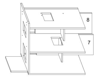
Insert C(wooden dowel) in No.5 panel top, joint it to No.6 panel, use A screw to lock No.6 panel on No.1 and 5 panel.
