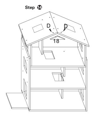
Use D screw to lock No.18 panel on No.15 and 17 panel.
