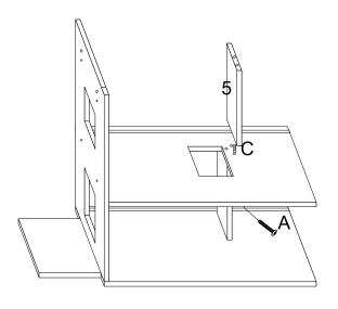
Insert C(wooden dowel) in No.5 panel bottom, joint it to No.3 panel, use A screw to lock No.5 panel on No.3 panel.
