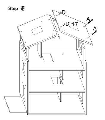
Use D screw to lock No.17 panel on No.16 panel, use A screw to lock No.17 panel on No.14 panel.
