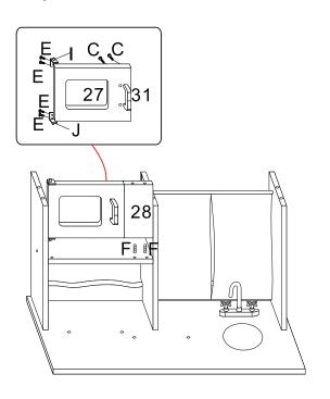
Use E screw to lock J(door pin) on No.27 panel up and down, insert No.27 panel on No.24 panel, use C screw to lock No.31 (handle) on No.27 panel, insert F(wooden dowel) in No.28 panel, joint it to No.24 panel.
