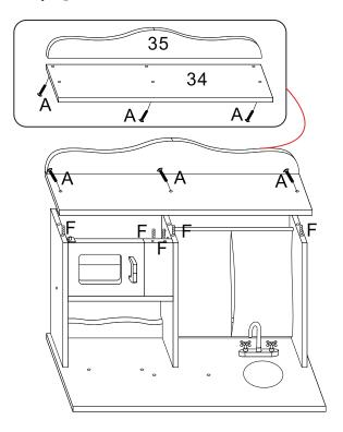
Use A screw to lock No.35 panel on No.34 panel, insert F(wooden dowel) in No.22,25,26 and 28 panel, joint it to No.34 panel,then use A screw to lock it.
