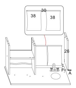
Insert F(wooden dowel) in No.26 panel, joint it to No.23 and 33 panel, across to No.38(fabric) to No.30(bar), joint it to No.25 and 26 panel, use A screw to lock No.26 panel on No.23 panel.
