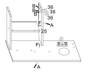
Use B screw to lock No.36(hooks) on No.25 panel, insert F(wooden dowel) in No.25 panel ,joint it to No.23 panel, insert F(wooden dowel) in No.24 panel rightside,joint it to No.25 panel, use A screw to lock No.25 panel on 23 panel.
