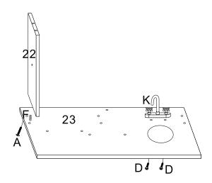
Insert F(wooden dowel) in No.22 panel, joint it to No.23 panel, use A screw to lock No.22 panel on 23 panel, use D screw to lock K(tap) on No.23 panel.
