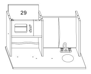
Insert No.29 panel in backside groove.
