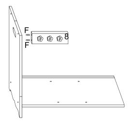
Insert F(wooden dowel) in No.8 panel leftside, joint it to No.5 panel.
