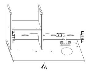
Insert F(wooden dowel) in No.33 panel bothside, across to No.25 panel hole, joint it to No.23 panel, use A screw to lock No.33 panel on No.23 panel.
