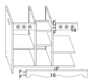
Insert F(wooden dowel) in No.14 panel leftside, joint it to No.12 panel, insert F (wooden dowel) in No.15 panel, joint it to No.5 and 6 panel.
