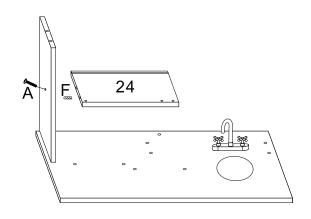
Insert F(wooden dowel) in No.24 panel leftside, joint it to No.22 panel, use A screw to lock No.24 panel on No.22 panel.
