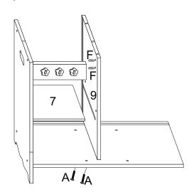
linsert F(wooden dowel) in No.8 panel rightside, joint it to No.9 panel, insert No.7 panel between No.5 and No.9 panel groove, use A screw to lock No.9 panel on No.6 panel.
