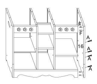
Insert F(wooden dowel) in No.14 and 15 panel rightside, joint it to No.16 panel, use A screw to lock No.16 panel on rightside.
