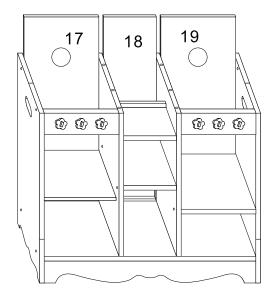
Insert No.17,18,19 panel in backside groove.
