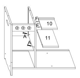
Use A screw to lock No.11 panel on No.9 panel, insert F(wooden dowel) in No.10 panel leftside, joint it to No.9 panel.
