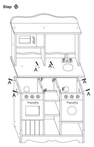
Insert F(wooden dowel) in No.9 and 12 panel top, joint it to the upper part of kitchen,then use A screw to lock it.
