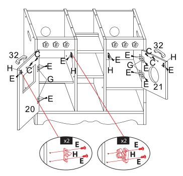
Use C screw to lock No.32(handle) on No.20 and 21 panel, use E screw to lock H(male door latch) on No.20 and 21 panel, use E screw to lock H(female door latch) on No.9 and 12 panel, use E screw to lock G(hinge) on No.20 and 21 panel.
