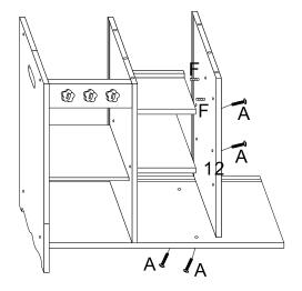
Insert F(wooden dowel) in No.10 panel rightside, joint it to No.12 panel, use A screw to lock No.12 panel on No.6 and 9 panel.
