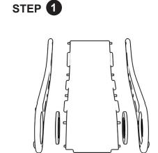
Place handrail A and B to the slide rail as shown (and insert washer inner 2).
