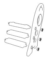
Fix steps to panel A as shown in illustration (C step to top rail) – tighten 3 nuts with locking tool.
