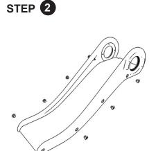
Secure handrails in place using the 8 small nuts and locking tool.
