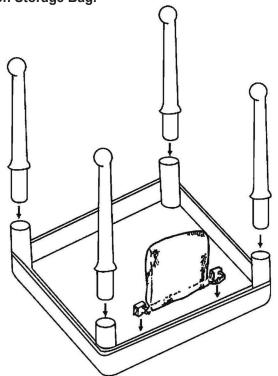
Smooth Top fits easily over base plate surface. To remove just lift up on sides.
