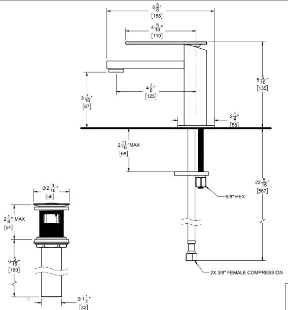
Ø 1-1/4" [32] Ø 1-1/2" [38] SPOUT: DRAIN: Ø 1-3/8" [35] Ø 1-3/4" [44] DIMENSIONS SHOWN TO THE NEAREST 1/16" [DIMENSIONS SHOWN TO THE NEAREST 1mm]
