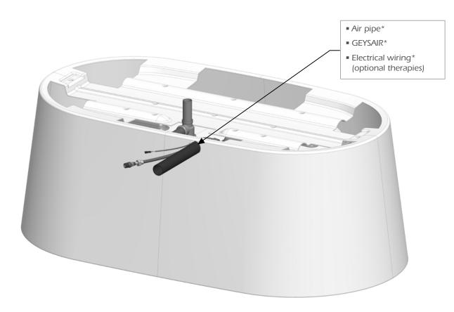
(\*): LOCATION SHOWN AS AN EXAMPLE MAY DIFFER ACCORDING TO THE POSITION OF REMOTE COMPONENTS AND LOCATION OF BATH. SEE PAGE 21 FOR INSTALLATION OF ISLAND TUB DRAIN® (ITD)
