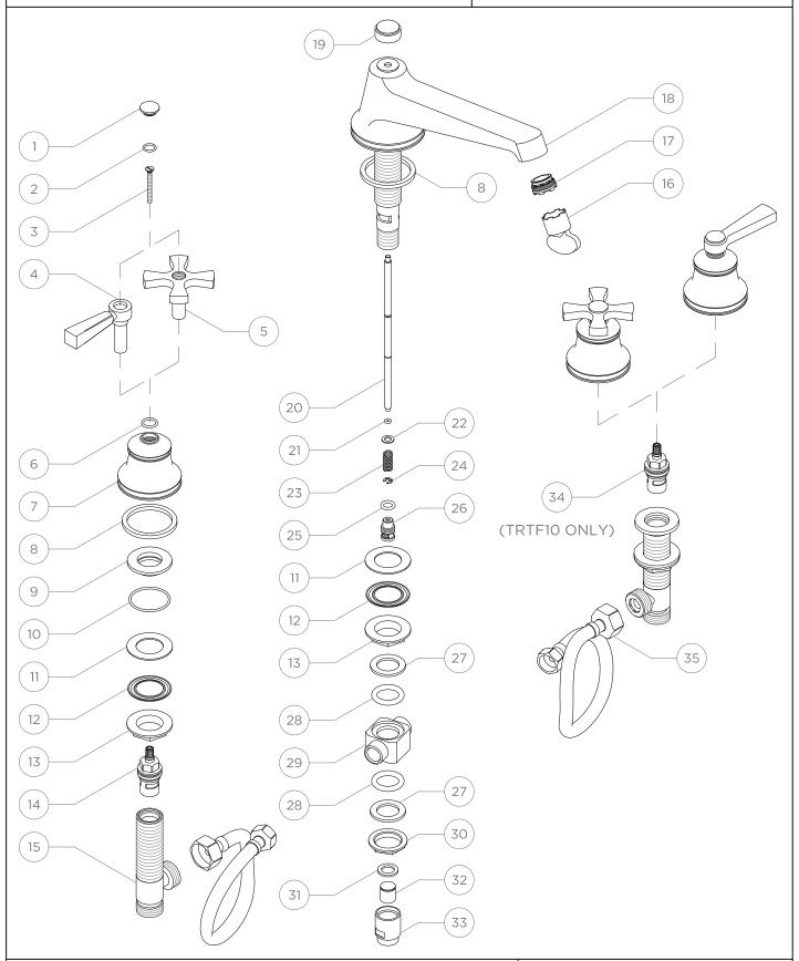
These guidelines have been prepared for the professional contractor to aid in the installation of: TRANSIT LOW PROFILE THREE HOLE DECK MOUNTED LAVATORY FAUCET WITH METAL CROSS HANDLES (STYLE No. TRTF0). AND METAL LEVER HANDLES (STYLE No. TRTF10).
