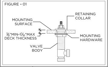
These guidelines have been prepared for the professional contractor to aid in the installation of: TRANSIT LOW PROFILE THREE HOLE DECK MOUNTED LAVATORY FAUCET WITH METAL CROSS HANDLES (STYLE No. TRTF01) AND METAL LEVER HANDLES (STYLE No. TRTF10).
