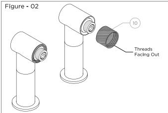
11. Securely tighten the union nuts (13) then thread the collars (10) back onto the valve body (14) to conceal the union nuts. See Figure - 03A.
