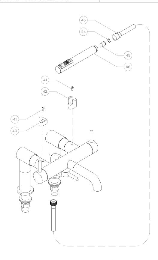
These guidelines have been prepared for the professional contractor to aid in the installation of: FLYTE EXPOSED DECK MOUNTED TUB FILLER WITH LEVER HANDLES AND HANDSHOWER (STYLE No. FLXT50).
