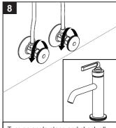
Turn on angle stops and check all connections for leaks.
