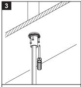
Use a screwdriver to tighten the ock nut.
