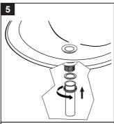
Install the drain tail piece to the drain plug.
