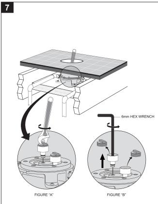
Turn off water supplies. With a wrench remove the center TEST PLUG as shown in Figure A. If the TEST PLUGS cannot be removed in one piece as shown in Figure A, the lower half will have to be removed using the supplied 6mm Hex Wrench as show in Figure B. Repeat step for the second TEST PLUG.
