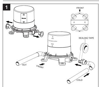
Sweat together Hot and Cold Supply assemblies. Apply sealing tape to threaded connections. With the maximum and minimum measurement in front, the hot supply is to be installed on the left inlet and the cold on the right as shown in the image above.
