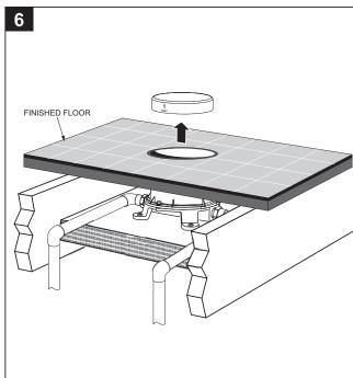
When you are ready to install the TUB FILLER cut the exposed part of the PLASTER GUARD flush with the finished floor. Be careful not to damage the floor.
