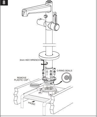
Remove PLASTIC CAP from bottom of the TUB FILLER. Before final installation, check that all sealing surfaces are clean and that the two O-RINGS are installed in the MOUNTING ADAPTER. Install the MOUNTING ADAPTER into the MANIFOLD MOUNTING BASE. Install the four MOUNTING SCREWS and WASHERS through the MOUNTING PLATE and into the MANIFOLD MOUNTING BASE. Do not tighten. Rotate the TUB FILLER right or left to align with Tub. Tighten MOUNTING SCREWS supplied with 6mm Hex Wrench to secure TUB FILLER.
