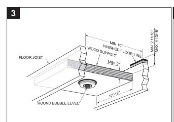
Adequate floor support is required. The WOOD SUPPORT must be a minimum of 2" (51mm) thick by 10" (254mm) wide. 2x6 lumber is NOT adequate for this application. WOOD SUPPORT must be located with in the MIN. and MAX. arrows that are marked on the front of the PLASTER GUARD.
