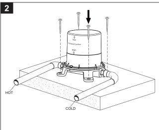
Locate the position on the wood support where the MANIFOLD MOUNTING BASE will be installed. Use the MANIFOLD MOUNTING BASE as a guide to mark the four mounting hole locations.Drill pilot holes if required. Secure the MANIFOLD MOUNTING BASE to the WOOD SUPPORT with SCREWS provided.Verify that the MANIFOLD MOUNTING BASE is level and then fully tighten SCREWS.
