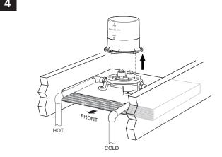
Finish all Hot and Cold supply connections to the MANIFOLD MOUNTING BASE .Loosen the two PLASTER GUARD SCREWS and remove the PLASTER GUARD. Make sure the two TEST PLUGS are tight, but do not over tighten. Turn on water supplies and test for leaks. Turn off water supplies. Replace PLASTER GUARD and attach with SCREWS.
