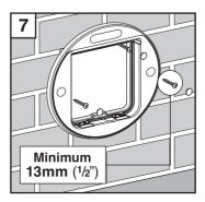
Position exterior frame on outside of wall and screw on using recommended screws. Finally, fit screw caps.
