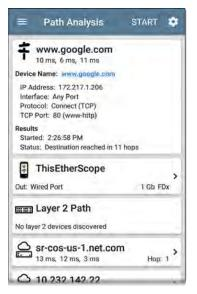
Like AutoTest, Path Analysis results are presented on cards. The top card shows the main test details, the second card shows information for the source device (your EtherScope nXG), and the following cards show the Layer 2 and Layer 3 Hops in the path, which are sequentially ordered.
