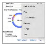
Touch blue links or the blue action overflow icon ••• at the bottom of the test results screens to run the HTTP TEST AGAIN, open another testing app, or Browse to the target address in your web browser. Captive Portal Connections
