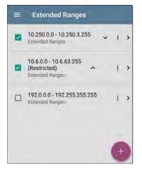
Check or uncheck the boxes to include or exclude an extended range from the current Discovery configuration. Unchecked Extended Ranges do not affect the default Discovery behavior in the current configuration, but they may be used in other Discovery configurations (like Community Strings and Credentials).
