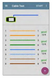
When a cable has no detected faults, "good" is shown next to each pair above the length measurement. Cable tests that detect a "split" or "open" in the cable also display the corresponding words.
