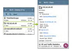
On the Wi-Fi Details screens, you can touch any blue linked name or address to open a Discovery or Wi-Fi app screen for the linked device. NOTE: Non-underlined links open in the same app (in this case Wi-Fi), and <u>under-</u> <u>lined links</u> open in a different app (in this case Discovery).
