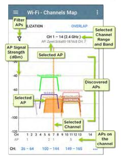
Touch the blue channel range selectors at the bottom to view a different channel range on the graph.
