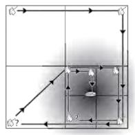
Go to one corner of your search area, and note the device's signal strength on the Signal graph.
