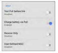
Test PoE before Link: By default, an AutoTest Wired Profile performs the Link test before the PoE test may be able to complete. Enable this setting to make your EtherScope complete the PoE test before the Link test. Enabling this setting forces PoE negotiation to be completed before establishing link, improving compatibility with some switches.
