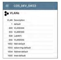
The VLANs Details screen also shows the description with each VLAN ID.
