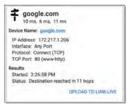
The top Path Analysis results card shows the path's Destination address at the top, followed by the three response times from the TCP Connect, Ping, or Echo tests. **Device Name**: Resolved DNS name or IP address of the destination entered in the settings
