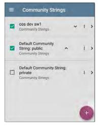
The EtherScope uses the checked strings in the order shown on this screen. If it does not receive a response from the queried device using one string, it sends the next string.
