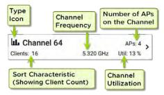
The lower left field displays the characteristic by which the list screen is currently sorted. In the image above, the Channels list is sorted by Client Count.
