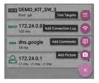
The Test Targets screen lists all of the defined and saved Test Targets. Checked boxes indicate the Test Targets that are enabled in the current Profile. Remember, Test Targets can be added to and used in any number of Wired or Wi-Fi Profiles.
