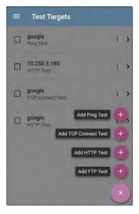
Touch any target's name, or add a new target, to open the test's settings, where you can enter a custom test name, target address, and thresholds.
