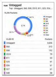
The VLAN test screen displays the real-time traffic the EtherScope detects on the top VLANs. Up to nine VLANs with the highest traffic are displayed as colored portions of the pie chart. The table on the lower part of the VLAN screen lists all the VLANs seen.
