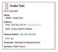
The top of the card shows the device type and icon (a Wi-Fi Controller with a **Failure or Error** status in the example image above).
