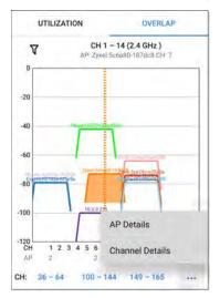
Touch the action overflow button ••• to open the AP Details or Channel Details screens for the selected AP or Channel.
