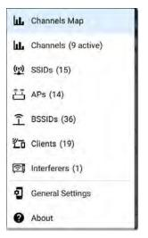
The Wi-Fi app's navigation drawer displays a real-time count (in parentheses) of each wireless component EtherScope has detected. Tap an option to open the corresponding screen.
