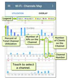
In the image above, the vertical light and dark blue bars show how much of the channel's capacity is being used by 802.11 devices and non-802.11 interference, with channel numbers on the x-axis and Utilization percentage on the y-axis.
