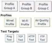
At the bottom level is a set of individual **Test Targets** that connect to network services, such as a web app or FTP site. A Test Target defines parameters including type, target URL/IP address, port number, and Pass/Fail thresholds. More complex tests, like HTTP, allow further Pass/Fail criteria, such as strings that must or must not be contained in the HTTP body. A Test Target can be added to and used in any number of **Profiles**.
