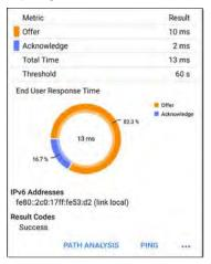
**Offer**: Time between when the EtherScope sent the discovery and received an address offer from the DHCP server
