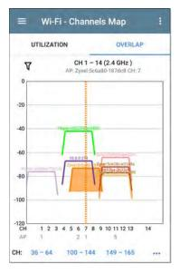
Touch an AP on the graph to select it and its primary channel. In the image above, the AP named "Zyxel:5c6a..." on channel 7 is selected.
