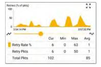
Retries (% of packets) graph: Plots percentage of transmitted packets that are retry packets
