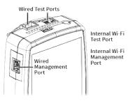
Either the top copper port or fiber port can act as the Wired Test Port, so in total, the EtherScope has *four* network interfaces: 1 Wired Test, 2 Wi-Fi Test, 3 Wired Management, and 4 Wi-Fi Management.
