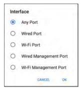
EtherScope must have an active network link on the selected port to run a Path Analysis. If **Any Port** is selected, available links are used in the order shown in the Interface dialog above.
