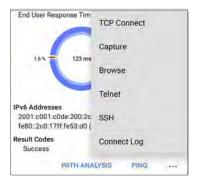
The additional actions available on the DHCP test screen include opening the Path Analysis, Ping/TCP, or Capture apps populated with the DHCP server address, browsing to the IPv4 address in the web browser, starting a Telnet or SSH session, or viewing the Connect Log.
