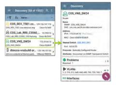
The available data and actions on the Details screens vary significantly depending on the device type, connections, and data the EtherScope was able to discover. In other words, only the discoverable information for each device is shown on the Details screen.
