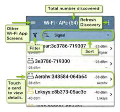
Like in AutoTest and other EtherScope screens, the icons in Wi-Fi analysis change color to indicate a Warning or Failure condition. The app also displays icons in Blue to indicate Problem-related information that does not constitute a warning or failure, and Green to indicate that a previous Problem has been resolved.
