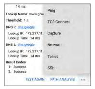
Touch blue links or the blue action overflow icon ••• at the bottom of the test results screens to run the DNS **Test Again**, open another app populated with the name and IP address of DNS 1, or **Browse** to the Primary DNS server in your web browser.
