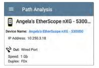
Beneath the EtherScope source card, the Hop cards show Layer 2 and Layer 3 devices determined to be in the Path.
