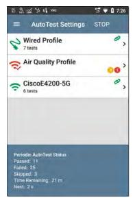
The Periodic AutoTest Status is summarized at the bottom of the AutoTest screens. Passes and failures are reported for each run of the entire Profile Group, rather than individual Profiles. Periodic AutoTests are skipped if the previous
