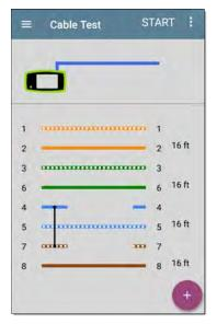
This unterminated cable test image shows a shorted cable between pins 4, 5, and 7.
