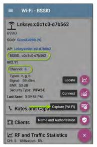
When the Capture app opens, filters are already set with the BSSID, Channel, and Channel Width from the Wi-Fi app.
