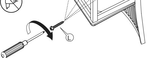
Assemble STRETCHER L/R to seat as illustration shown.To ensure chair level, assemble the chair on flat & soft surface.Tighten all screws & bolts using Allen Key while making sure that the unit remain level.Paste the M under the leg as shown on drawing.
