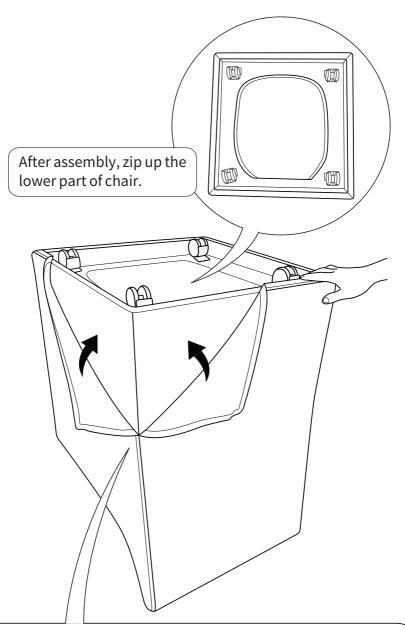
Pull the fabric on the upper part of chair straight and keep its edges flat before sticking it to the bottom of the lower part.
