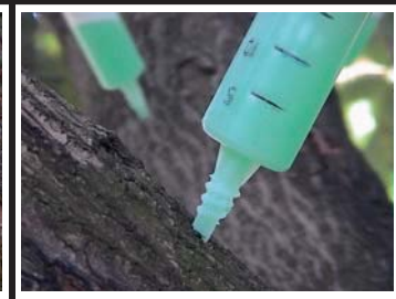
PIC 4 20mm extended nozzle tip requiring only a 4.2mm hole (wood dependent).
