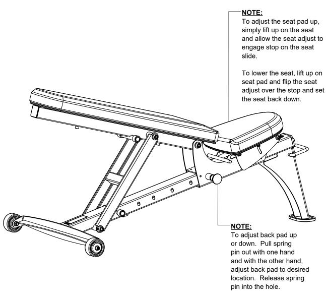
**NOTE:** Back pad adjustments in 15 degree increments. Flat, 15, 30, 45, 60 and 75.
