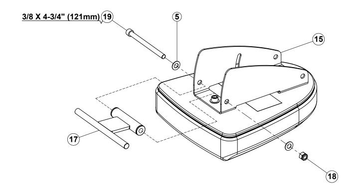
NOTE: SECURELY tighten bolt connection, then back nut off 1/4 turn. Part should rotate freely.
