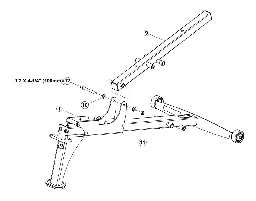
NOTE: SECURELY tighten bolt connection, then back nut off 1/4 turn. Part should rotate freely.
