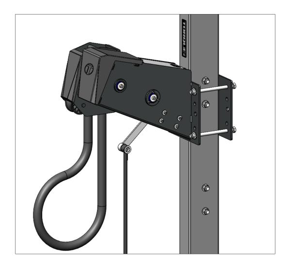
With the included "BACKING PLATE" the XERT can be mounted to any tube without holes like shown. Maximum tubing width or height (depending on if mounting to a horizontal or vertical tube is 150 mm (6 inches).
