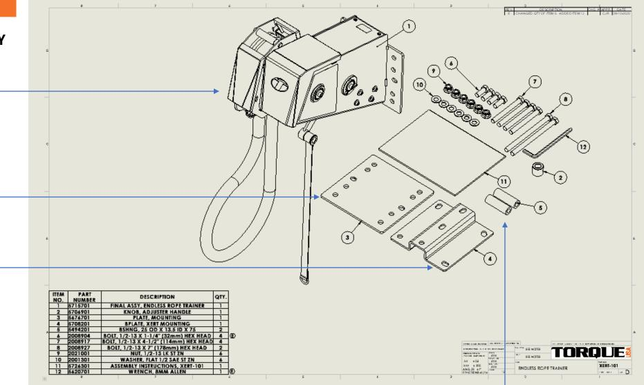
BUSHINGS ARE USED IN CASES LIKE THE X-LAB EDGE WHEN MOUNTING INSIDE A U-BRACKET
