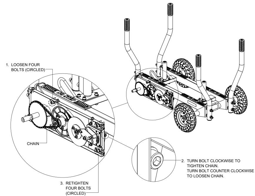
The chain tension on TANK is pre-set at the factory. However, if the chain becomes too loose or is too tight, then please follow the steps in numbered order to adjust.
