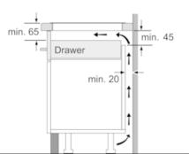
Measurements in mm
