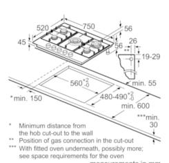
measurements in mm
