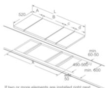
If two or more elements are installed right next to one another, one or several installation kits a required (2 elements 1 installation kit, 3 elements 2 installation kits, etc.).
