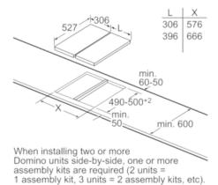
Measurements in mm
