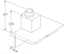
If a back panel is used, the design of the appliance must be considered. measurements in mm
