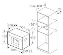
Bean and water containers are removed from the front. Recommended installation height 95-145 cm. measurements in mm
