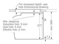
measurements in mm
