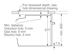
measurements in mm
