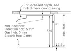
measurements in mm
