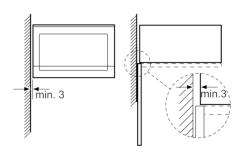
Measurements in mm
