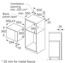
\* 20 mm for metal fascia measurements in mm
