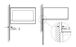
Measurements in mm
