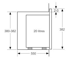
measurements in mm
