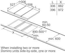
When installing two or more Domino units side-by-side, one or more assembly kits are required (2 units = 1 assembly kit, 3 units = 2 assembly kits, etc).
