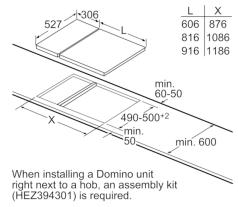
Measurements in mm
