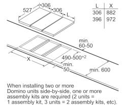
Measurements in mm
