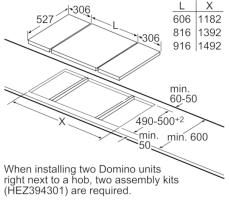
Measurements in mm
