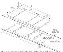
If two or more elements are installed right next to one another, one or several installation kits are required (2 elements 1 installation kit, 3 elements 2 installation kits, etc.).
