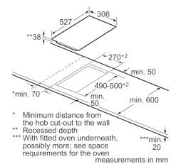
Picture for the table Domino combination possibilities with corresponding devices and cutout dimensions
