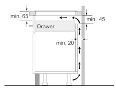
Measurements in mm 3/3
