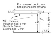
measurements in mm
