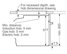
measurements in mm
