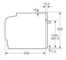
measurements in mm
