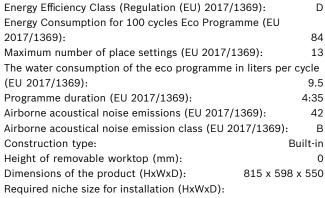
815-875 x 600 x 550 Depth with open door 90 degree (mm): 1150 Yes - all from front Adjustable feet: Maximum adjustability feet (mm): Adjustable plinth: both horizontal and vertical Net weight (kg): 43.830 Gross weight (kg): 46.0 Connection rating (W): 2400 Current (A): 10 Voltage (V): 220-240 Frequency (Hz): 50; 60 Length of electrical supply cord (cm): 175 GB plug Plug type: Length inlet hose (cm): 165 Length outlet hose (cm): 190 EAN code: 4242005270293 Full-integrated Installation type:
