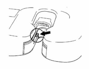
WHILE LOOKING INTO THE TYING APERATURE AND HOLDING THE TIE HOLDING ARM, CONTINUE PUSHING THE TWIST TIE RIBBON UNTIL IT APPEARS ABOUT 1/8" INTO THE TYING APERATURE. MACHINE IS NOW LOADED.
