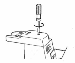
LOOSEN THE TOP COVER FIXING SCREW BY USING A SCREWDRIVER AND TURNING SCREW IN A COUNTER-CLOCKWISE DIRECTION.
