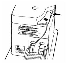
REMOVE THE TWIST TIE RIBBON FROM THE MACHINE BY PRESSING THE TIE HOLDING ARM AND PULLING BACK ON THE MATERIAL.
