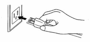
MAKING SURE THE ON/OFF SWITCH IS IN THE OFF POSITION, PLUG MACHINE INTO POWER OUTLET CHECKING THAT OUTLET IS OF THE CORRECT VOLTAGE.
