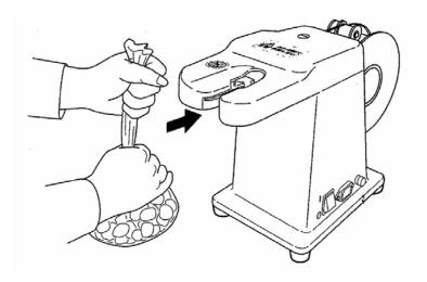
SQUEEZE THE TOP OF THE BAG OR BUNDLE TO BE TIED AND INSERT IT INTO THE TYING APERATURE OF THE MACHINE. HESITATE WHILE THE MACHINE COMPLETES THE TIE AROUND THE PRODUCT. UPON COMPLETION OF THE CYCLE, REMOVE THE TIED AND PRODUCT AND THE MACHINE IS READY FOR THE NEXT CYCLE.
