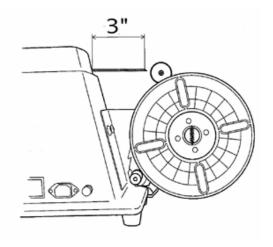
WHEN FINISHING A SPOOL OF TWIST TIE RIBBON IT IS IMPORTANT THAT APPROXIMATELY 3" OF RIBBON REMAINS OUTSIDE THE MACHINE AND IS REMOVED. DO NOT FEED THIS INTO THE MACHINE AS IT MAY CAUSE JAMMING.
