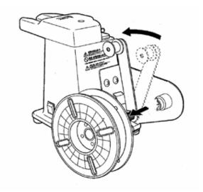
REMOVE THE ROLL OF TWIST TIE FROM THE RIBBON SPOOL MANDREL BY LOOSENING THE KNOB AND MOVING THE STOPPER PLATE TO THE CENTER OF THE TWIST TIE RIBBON SPOOL. TIGHTEN THE KNOB SO THE STOPPER PLATE IS EVEN WITH THE RIBBON SPOOL MANDREL. TO INSTALL A NEW SPOOL OF TWIST TIE RIBBON ON THE MACHINE FOLLOW INSTRUCTIONS IN SECTION 5.
