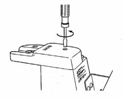
WHILE HOLDING THE TOP COVER IN PLACE, TIGHTEN THE TOP COVER FIXING SCREW.
