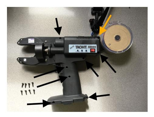
4. Remove the two, silver screws that are behind the twisting propeller.
