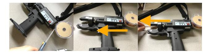
3. Remove the eight, black screws that hold the frame together.
