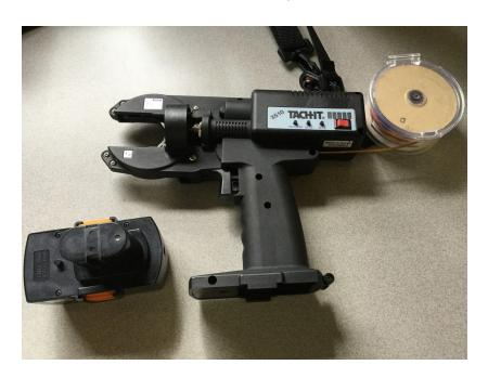
2. Remove material from the gun by cutting it between the back of the gun and the spool, and pushing it toward the *front* of the gun. Do NOT pull it backwards out of the gun as this will put undue wear on the rollers.
