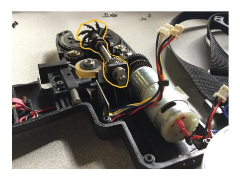
8. Remove the screw at the rear of the shaft, take of the encoder, use a flat head screwdriver to remove the c-clip, remove the washer, and push the brass bushing towards the rear to pull it off. (Note that the encoder is "keyed" with a flat side on part of the inside circle that goes onto the shaft. When putting the encoder back, make sure the flat sides match up with each other. IT IS VERY IMPORTANT THAT THE ENCODER IS NOT BENT. IF IT IS, THE GUN WILL NOT WORK PROPERLY)
