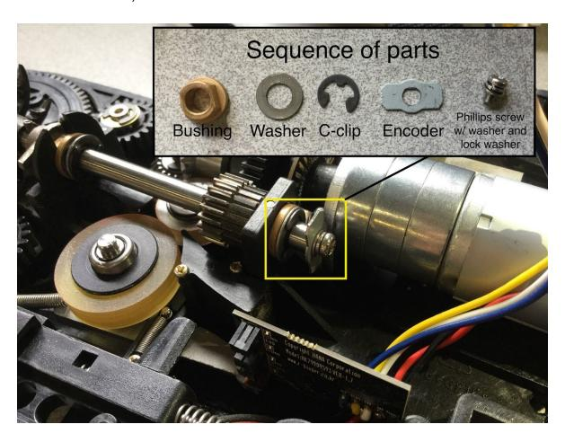
9. There are four items that hold the front of the shaft in place. In order, from rear to front, there is a c-clip, washer, wave spring washer, and brass bushing. Remove the c-clip, and move the other three items towards the rear.
