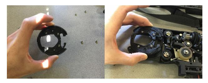
13. After replacing the carrier arm and propeller shaft (Reverse of steps 7-9), prop the gun upside down, resting against your body on the edge of the your work bench. Place the top of the body flat on the table, perpendicular to the half that is resting against you. Reconnect the three plugs (See step #6), and then replace the screws (See steps 3-5). Feed some material into the gun and test it to make sure it is functioning properly.
