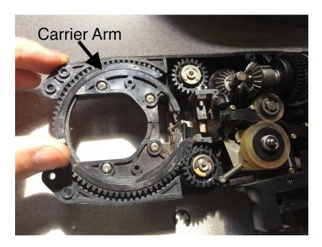
11. Sometimes a wire or other piece of debris will jam inside the circular carrier arm and/or cause it to come off of its track. If this happens, remove the four screws that hold the carrier track in place. Note that the track is comprised of two pieces (top and bottom) and that there are nuts on the other side of the screws. Note that the longer ones are towards to rear of the gun, and the shorter ones are towards the front of the gun.
