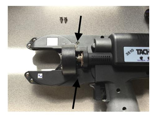
5. Remove the four, silver screws that are on the very front of the gun, two on top, two on bottom. Note that there are nuts on the back side that will fall to the table when the screws come out.
