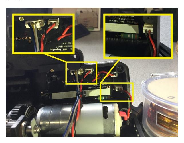
7. Some jams will require you to remove the shaft that spins the twisting propeller. First, locate the shaft.
