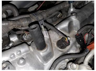
2. Remove the hose that connects the supercharger inlet (snout) to the valley pcv, connect the supplied 3/8 hose to the valley pcv and lay to the side, then put the 3/8" vacuum cap on the supercharger port.
